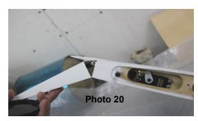
Fit servo horn to 8911 flap servo. Centre servo and do setup for travel with TX.
